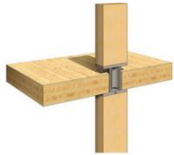
CLT floor slabs with glulam columns and steel connectors
